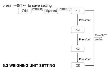
Keep pressing **ON**, when **Unit** is shown ,Then operation as blow:
