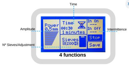
Adjustment of 4 different parameters with only one command and LCD screen which allows access to all information during sieving.
