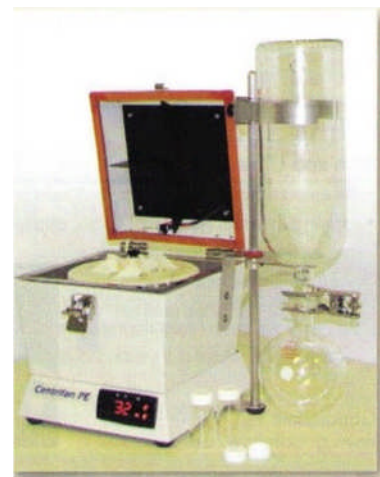
Centrifan™ PE streamlines final dry-down into Scin vials and Eppi tubes.
