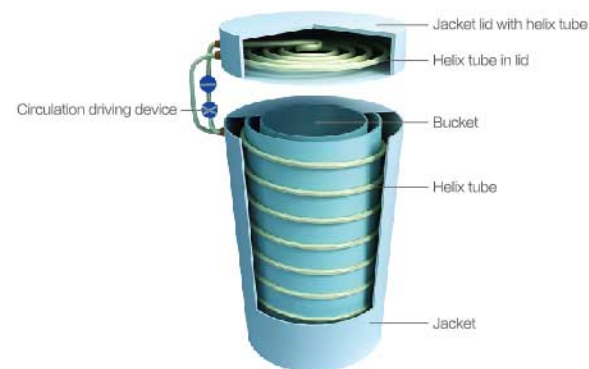
Diagram for helix tube multi-point isothermal technology
