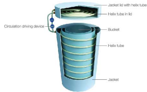
Diagram for helix tube multi-point isothermal technology
