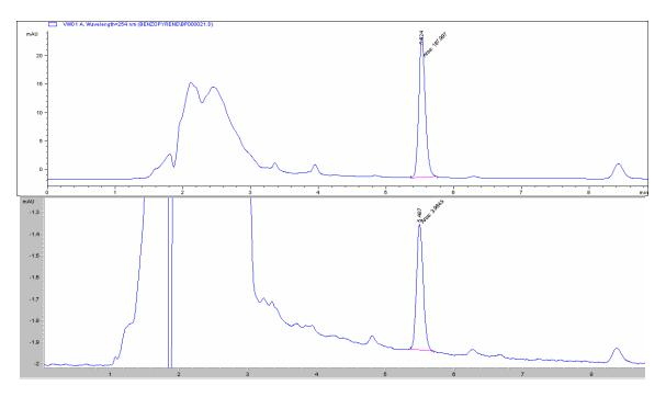
Upper figure: tap water spiked with 2.5 ppb benzo(a)pyrene, inject 20 mL Lower figure: tap water spiked with 25 ppt benzo(a)pyrene, inject 40 mL
